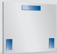
Hood inner panel with local patchworks
